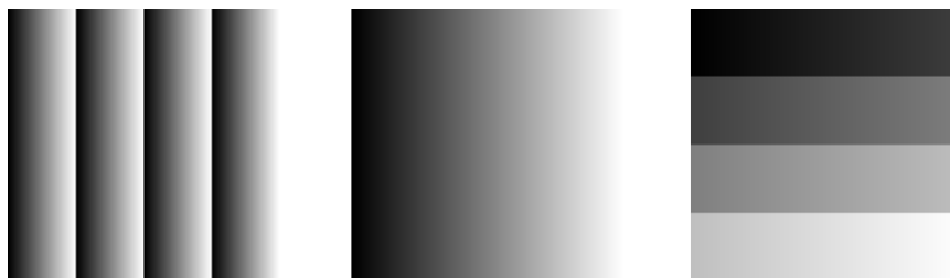
Figure 4.21: Ramp test images: 8 bit output (left), 10 bit output (middle), 12 bit output (right)
