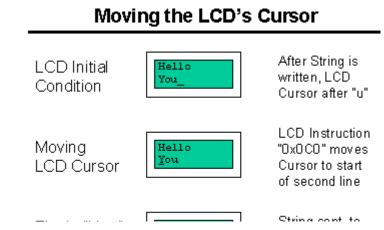
Cursor to Display" instruction is used. For this instruction, bit 7 of the instruction byte is set with the remaining seven bits used as the address of the character on the LCD the cursor is to move to. These seven bits provide 128 addresses, which matches the maximum number of LCD character addresses available. The table above should be used to determine the address of a character offset on a particular line of an LCD display.
