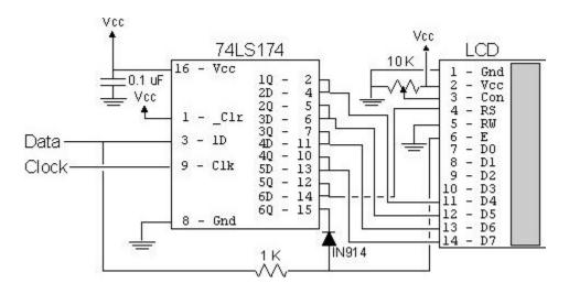
I normally use a 74LS174 wired as a shift register (as is shown in the schematic diagram) instead of a serial-in/parallel-out shift register. This circuit should work without any problems with a dedicated serial-in/parallel-out shift register chip, but the timings/clock polarities may be different. When the 74LS174 is used, note that the data is latched on the rising (from logic "low" to "high") edge of the clock signal.
