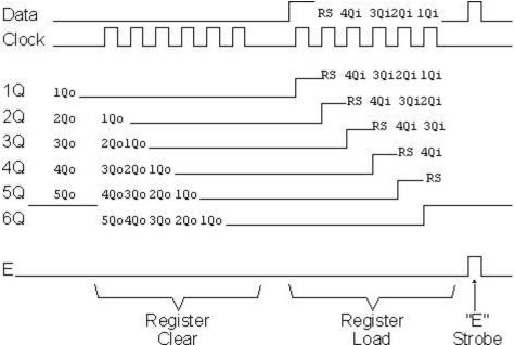
to be cleared before it can be loaded and the two wire operation requires more than twice the number of clock cycles to load four bits into the LCD.
